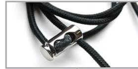
**8-wire Neckloop:** This cord hangs the Quattro 4L around your neck like a necklace. This is an 8-wire loop that connects to hearing aids or cochlear implants with t-coils, delivering sound directly through the hearing aids or cochlear implants when they are in t-coil mode.
