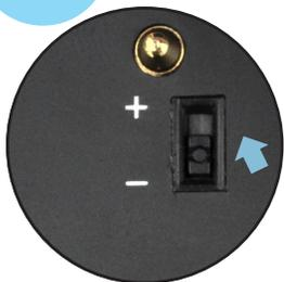
**STEP 1:** Use the tip of a pen to move the battery engagement +/- switch into the + position on the Quattro 4L.
