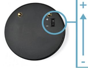
**Battery Engage Switches:** There is a battery engage switch on the Quattro 4L unit. This switch **MUST** be in the **+** position on the Quattro 4L for the unit to function. By switching to the **-** position, the battery is disengaged from the circuit. This switch does **NOT** need to be put in the **-** position; its purpose was to protect the integrity of the battery during storage.
