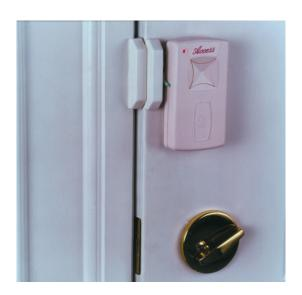
Never be surprised by someone entering through a door (or window) unexpectedly. This unit is comprised of two small magnetic contact bars and a transmitter. When the door or window is opened, the two bars lose magnetic contact, triggering the transmitter. The transmitter then sends a signal to the receiver, and depending on which receiver you are using, you will be alerted by a vibration or a strobe light.
