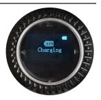
**STEP 5:** QUATTRO 4 is charged when screen indicates 100% and battery icon shows full.
