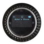
STEP 4: When the device name appears on the QUATTRO 4 screen, it is paired and connected.
