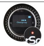
**STEP 4:** Charging... appears on the screen, and the red light is on.
