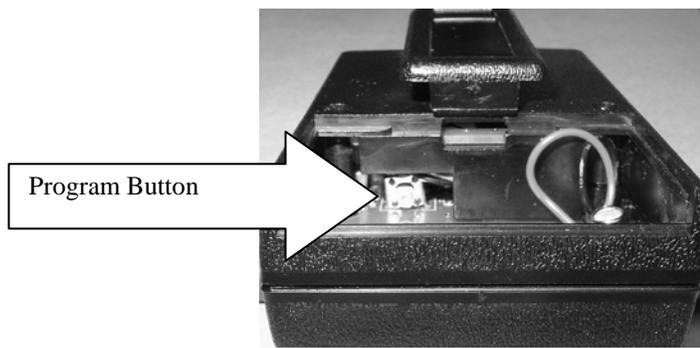
3. Press and hold the PROGRAM button. While pressing the program button, turn the Omni Pager on, hold on for 8 – 10 seconds and then release the PROGRAM button. This will erase all codes in the Omni Pager's memory.
