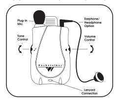
Turn on the POCKFTALKER® ULTRA by turning the Volume Control counter-clockwise. The red "on" indicator light on the top of the unit should be lit.
