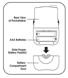
into place over the black ribbon, being careful to observe correct placement of (+) and (-) terminals.
